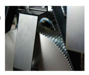
The implementation of a belt drive makes the design much simpler and, as a result, much easier to manufacture and assemble. Tolerances are less critical because the flexible timing belt will compensate. Because of the looser tolerances, parts are less expensive. An added benefit of this design is that servicing is much easier as well.
